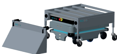
MiR100™/MiR200™ with ROEQ C300 approaching the Docking Station.
